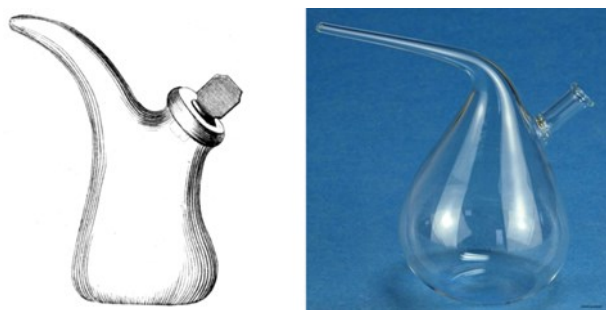
Fig. 5. Dropping bottle according to Schuster , on the left in one of the oldest illustrations according to J. A. Bucher's book Reperitorium für die Pharmazie, VI. Band. (Nürnberg, 1819), on the right the present-day form
